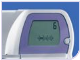
The Test Stick Symbol will flash while the Monitor is reading a Test Stick
